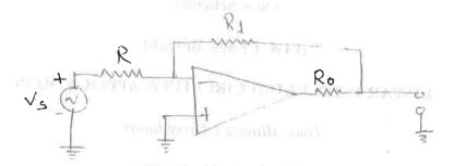
(d) For an op-amp the values of  $R_F$  and  $R_1$  are  $100 \, \mathrm{k}\Omega$  and  $1 \, \mathrm{k}\Omega$  respectively. It is an inverting amplifier with intput offset voltage drift of  $14 \, \mu \, \mathrm{V/^\circ C}$  and input offset current drift of  $0.5 \, \mathrm{nA/^\circ C}$ . The amplifier is nulled at 25°C. Evaluate the error voltage and the output at 45°C if input is TmVdc.
